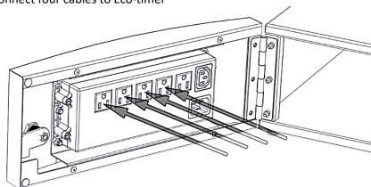
Connect the power cord to a wall socket and rout through the rear grommet, then plug into Eco-timer IEC C20 socket (USA) or IEC C14 (rest of world)
