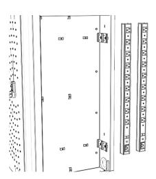
Unscrew the mounting plates and move to the adjacent panel
