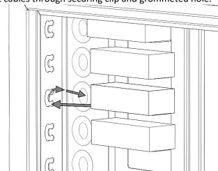
Rout device cable through grommet, adjust length and secure in the cable catch (depending on whether the device's power socket is on the LHS or RHS)
